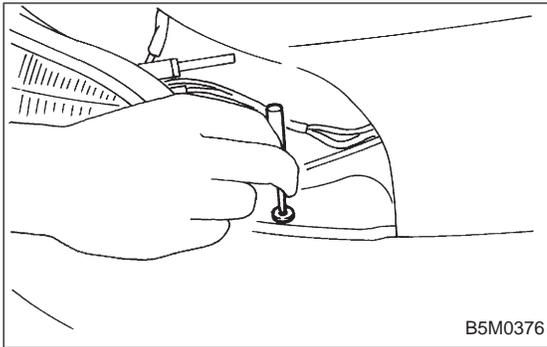
8) Remove clips from both sides of front bumper.
